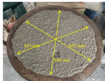
Fig. 2. SCC flowability measurement
